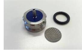
2. Remove the Adapter and the Cylindric House using the Nipple Key and clean the parts with Miris CLEANER. Rinse with distilled/deionised water. If the Adapter and Cylindric House are hard to separate, let them soak in Miris CLEANER for a while and try again.
