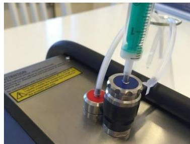
Figure 24. Leave the syringe on the inlet during the measurement.
