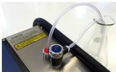
Figure 27. Inlet Pressure Guard (IPG)
