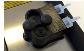
3. Reassemble the Filter House Restrictor and Stop Cover House Restrictor and attach to the instrument.
