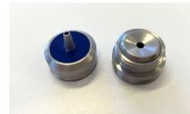
3. Use the Nipple Key provided to unscrew the outlet from the instrument. Open the outlet, carefully remove the gaskets by using a toothpick or similar. Clean the parts using Miris CLEANER. Rinse with distilled/deionised water.
