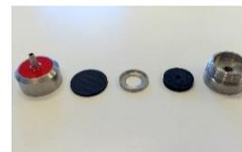
4. Assemble the outlet and mount it onto the instrument. Put back the waste tube and inject distilled/deionised water as described in Cleaning at the end of the day.
