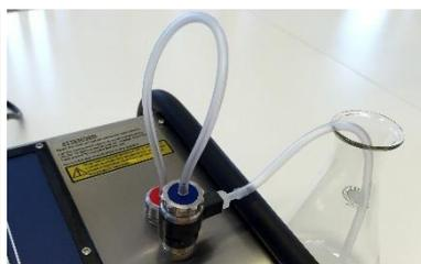
Figure 60. Inlet Pressure Guard (IPG).
