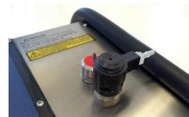
7. Attach the Filter House on the Adapter and connect tubes to the vent on the side of the IPG, and the outlet. Test the mounted IPG by injecting a few syringes with distilled water. At pressures below 3 bar (normal injection) fluid should not pass via the vent on the side of the IPG with a squeaky sound. Also make sure it is not leaking. If water is leaking, tighten the Adapter and test again.
