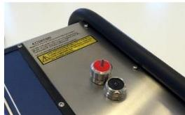
5. Remove the outlet using the Nipple Key, separate the gaskets and clean the parts using Miris CLEANER. Rinse with distilled/deionised water, reassemble the outlet and attach to the instrument. See Figure 9 for a detailed picture of the outlet.
