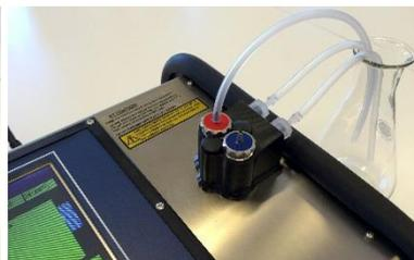
Figure 5. Cuvette Pressure Guard (CPG).
