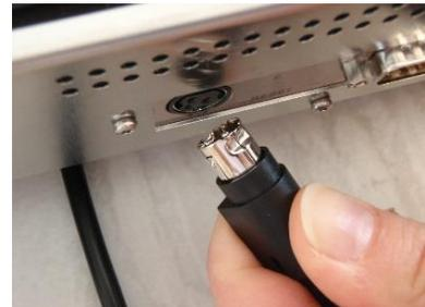
2. Keep the cover pulled back while you insert the plug. Attach the instrument to a power source and turn on the instrument by pressing the on/off button. The licensed application software will automatically start when the instrument is turned on.
