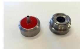
6. Place the Adapter on the Valve Case and put the Nipple Key in the cuts on the side of the Adapter, while rotating the Cylindric House in the opposite direction to tighten. Position the Cylindric House with the vent to the side of the instrument.
