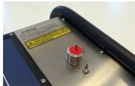
4. Attach the Valve Case to the instrument.
