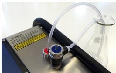
Figure 4. Inlet Pressure Guard (IPG).
